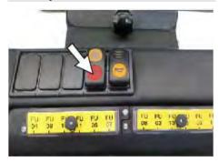
→ Switch on manual filter shake off.
