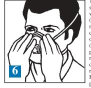
The seal of respirator on the face should be fit-checked prior to wearing in the work area. (a) Cover the front of the respirator with both hands, being careful not to disturb the position of respirator. (b) Inhale sharply. A negative
