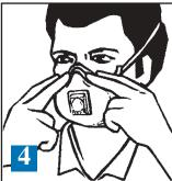
Using both hands, mould metal nosepiece comfortably to shape of nose. Pinching the nosepiece using one hand may result in less effective respirator performance.
