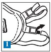
Thread top elastic strap through top buckles. Repeat for bottom strap and buckles. Place the bottom elastic strap around the head just below the ears. Untwist the strap.
