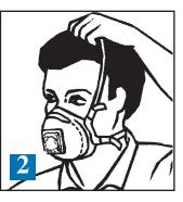
Place the top elastic strap around the head, above the ears. Untwist the strap.
