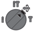
Vario-Lock position for adjustment of the chiselling position The mode selector switch 13 does not latch in this position.
